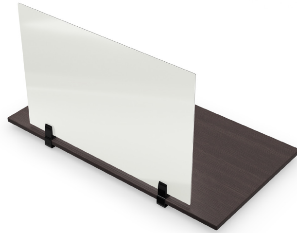
Setup B supports screen installation with space gap (5/8") above worksurface. Assemble bracket with the screen grip section attaching to the top side of the adjustable table top clamp.
