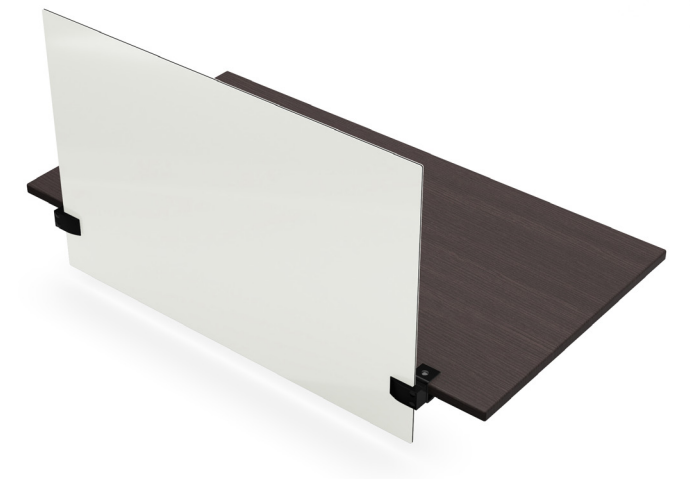
Setup D supports divider screen installation with benefit of a modesty panel. Rotate screen clamp 90° prior to attachment. Then assemble bracket with the screen grip section attaching to the exterior side of the adjustable table top clamp. Note: Available in 18" x 24", 18" x 36", 24" x 24", 24" x 36" sizes.
